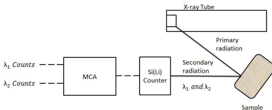
Fig.2.1 Schematic representation of spectroscopy with energy dispersive system.
