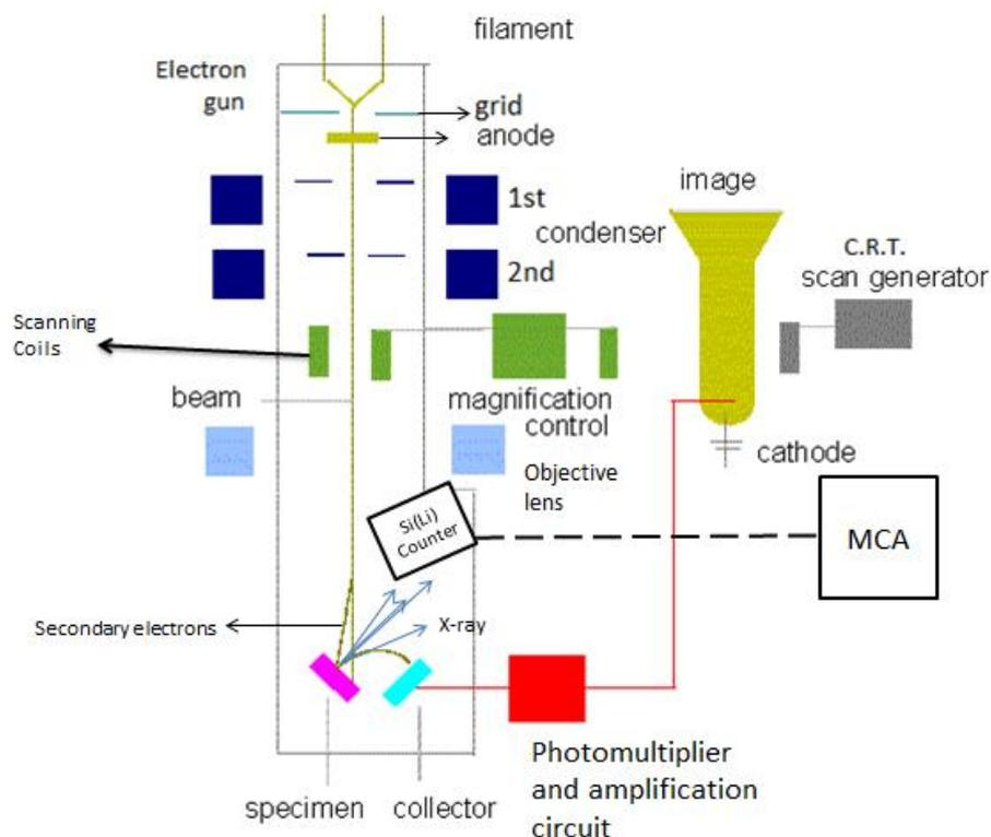
Fig.2.2 Schematic of a scanning electron microscope (SEM)
