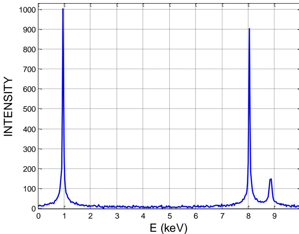
Fig.2.3 Elemental analysis of copper powder with energy dispersive system (EDS).
