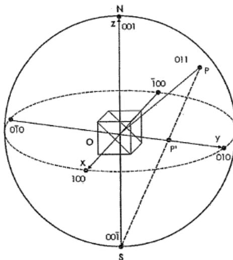
The northern hemisphere is projected onto the equatorial plane to obtain the stereographic projection. This is called as the “ $001$  standard projection of a cubic crystal”. Only the information from the northern hemisphere is needed since the southern hemisphere is a duplicate with negative indices.
