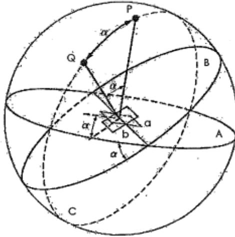
Figure 4.1. Spherical projection of the crystal
