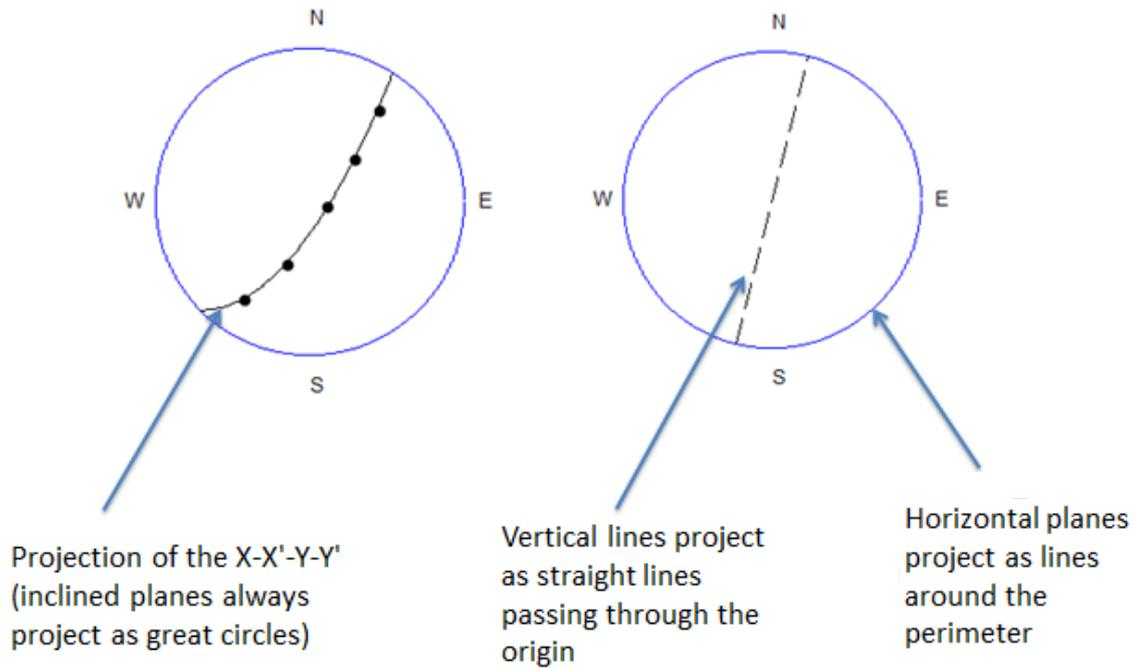
Fig.3.4 Top view of the projection plane.
