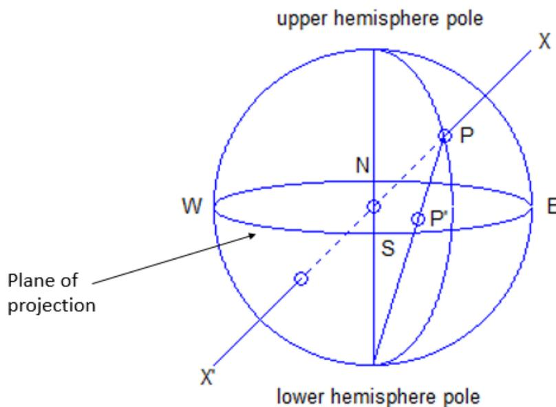
Fig.3.1 The stereographic projection of the line X-X'.
