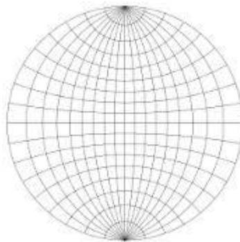
If the sphere is tilted such that the North South axis becomes horizontal, then the projection shown at the right in the above figure is called as the “Wulff net”. In this projection, lines of latitude on the reference sphere project to the horizontal arcs shown. The lines of longitude (great circle) project to the vertical arcs from the North Pole to South Pole. In most cases, a
