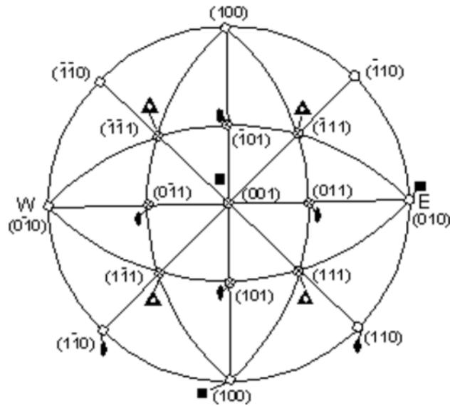
Figure 4.2 The 001 standard projection of a cubic crystal: a useful aid as it shows clearly the relative presentation of all the important plans in a crystal.
