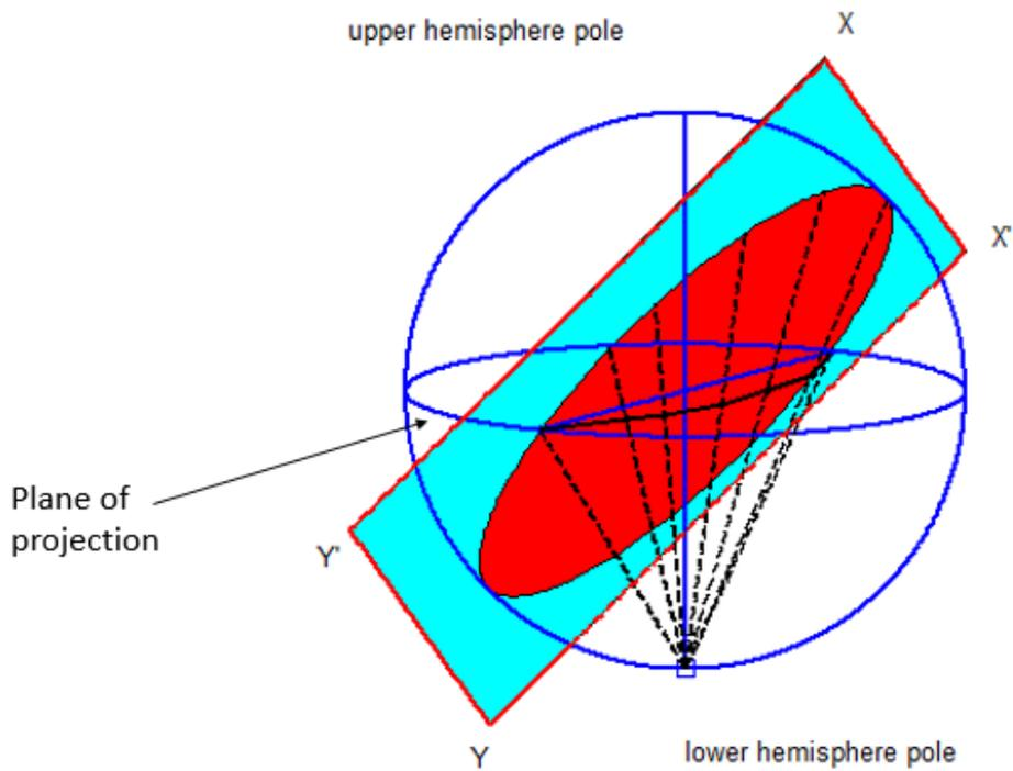
Fig.3.3 The projection of the plane X-X'-Y-Y'
